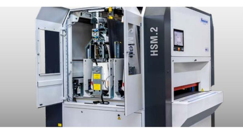
The HSM New Edition is the automatic surface sanding machine for **small** and **medium-sized craft and industrial** companies. Whether effect sanding, cross sanding, lacquer or high-gloss sanding, whether panels, solid wood or veneered workpieces - the Heesemann HSM New Edition is the optimally matched sanding machine for the craft! In its standard configurations with two, three or four units, the HSM New Edition is ideally prepared for all typical applications.
